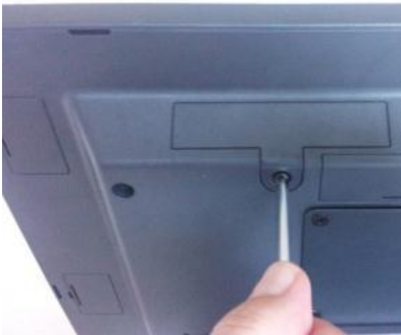
HDD access panel
