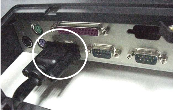
a. Connect the DB-9F cable.
