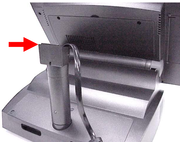
e. Install the top of the pole display to the support pole.
