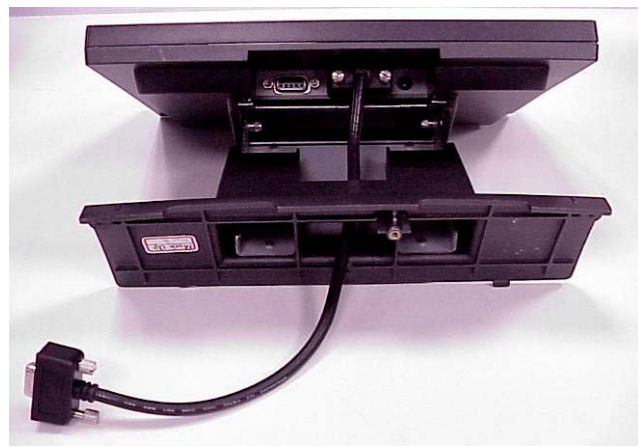
b. Connect the male head of the VGA cable to the second display.
