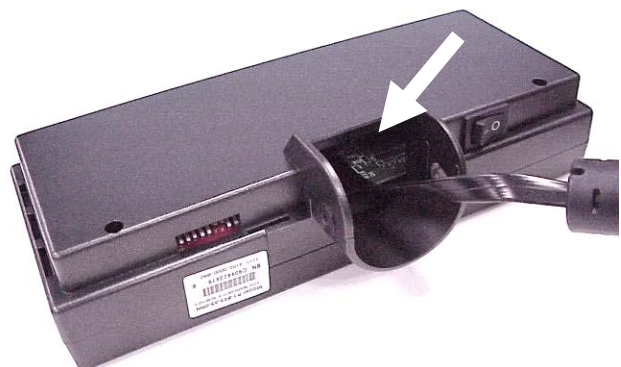
f. Connect the RJ45 connector into the jack of the customer display.
