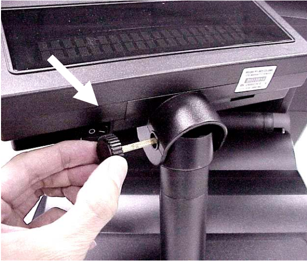
g. Insert the screw into the hole of the connection kit.
